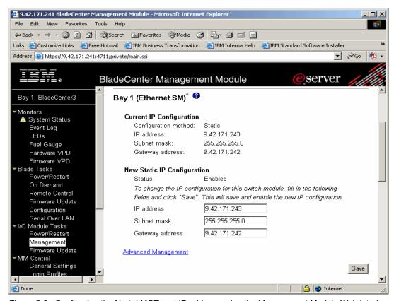
Figure 5-2 Configuring the Nortel MGT port IP address using the Management Module Web interface
